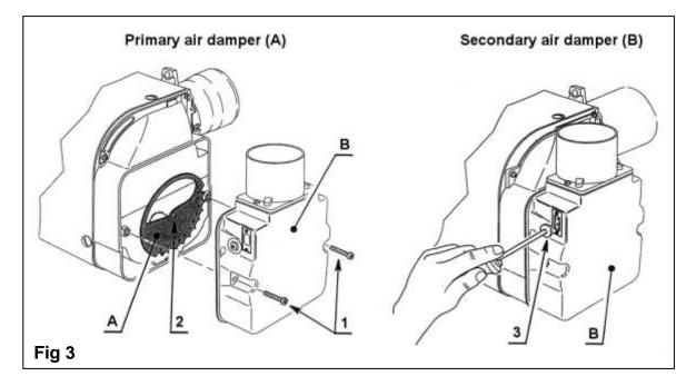
To set the primary air damper (**A**), remove the secondary air damper (**B**) by loosening the screws (1). Loosen the primary air wheel screw (2) and rotate the primary damper to the required position. Retighten the screw and replace the secondary damper.
